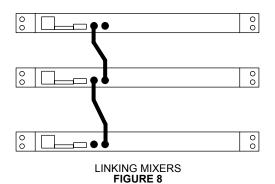
As long as the link jacks of all mixers are connected (out-to-in, sequentially, leaving one Link In and one Link Out jack unconnected), the automatic mixing functions will be shared by all units. All input signals appear at all linked mixer outputs. There is no master/slave relationship.
